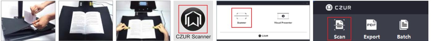
3. When scanning glossy materials like magazine, coated paper, photo, switch the anti-reflection side lights ON and main lights OFF for best effect.
