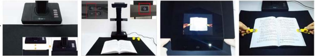
1. Spread the black document pad under the scanner's head. Ensure that the black document pad aligned with the device without any gap.
